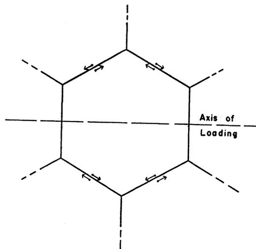
FIG. 2. Illustration of slipping at grain boundaries in a two-dimensional lattice. The arrows give the directions of slip.
